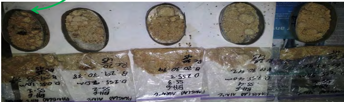
Moisture contents of disturbed soil samples
